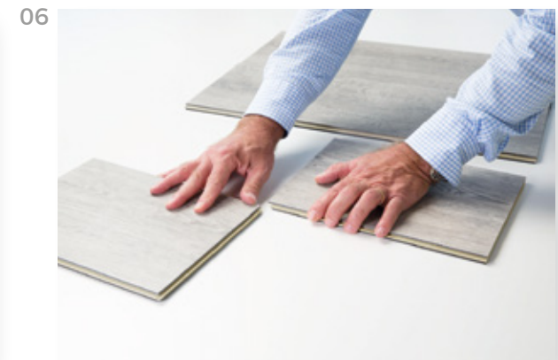
Continue sliding until the planks are fully separated
